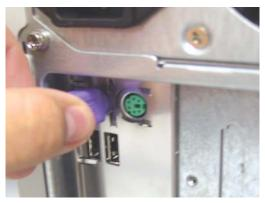
Attach the DKVM-2K's built-in mouse cable to the PS/2 mouse port located on the back of your computer case.
